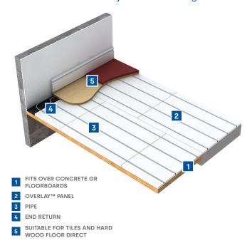
Because of their nominal 18mm thickness the panels can be simply installed on top of the existing structural sub-floor in a brick like pattern with minimal disruption to floor height. Another benefit is that most floor coverings such as ceramics and natural or engineered timber can be applied directly to the panel.
