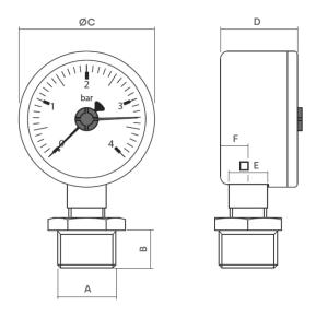
The gauge has been specially selected to cover the various pressure ranges encountered in heating systems which fall within 4 bar, 6 bar and 10 bar. By selecting the appropriate gauge the pointer has maximum rotational movement giving a sensitive response as the pressure increases or decreases. They can be installed in isolation or as part of a valve or other multi part equipment including;
